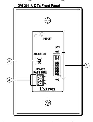
Figure 2-12 — DVI 201 Tx front panel connectors
